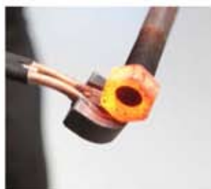
Releasing of rusted bolts
